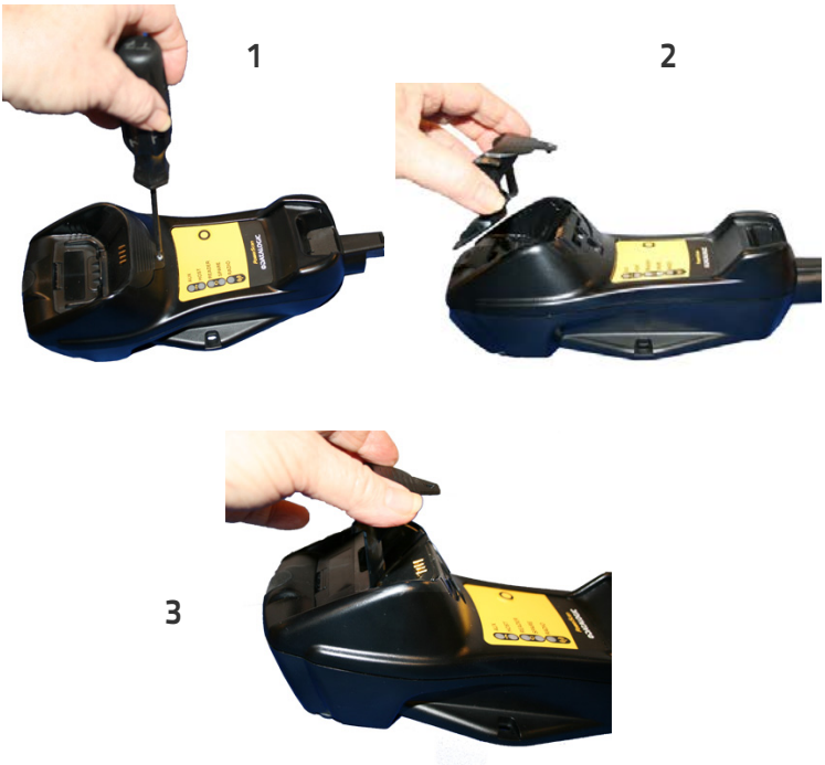
Figure 2. Changing the Bracket
