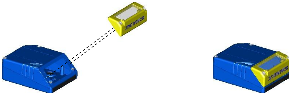
Figure 16 - Mounting a GFC-2020 Deflection Mirror
