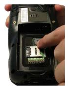
6. First insert the bottom and then the upper (contacts) side of the battery pack into the slot. Press until the battery latch clicks twice.
