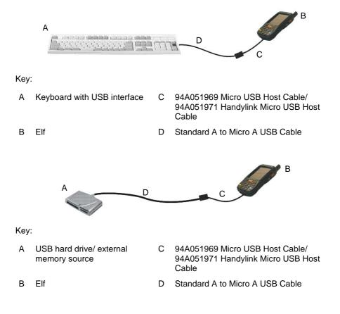
Connect the Single Slot Dock to the peripheral by means of a Micro-A USB cord, or use a Micro-A to Std-A receptacle USB adapter such as Datalogic 94A051969 (together with a standard USB cable if needed).
