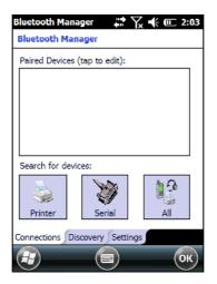
2. Search for available Bluetooth® devices by tapping the button for the type of device you want (Printer, Serial or All) or tap the Discovery tab and then tap the Discover button to skip this step. The Elf will search for Bluetooth® devices within range.
