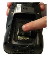
4. Insert the SIM card with the contacts downward:
