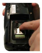
5. Lock the card into place by pushing the cardholder down and then shifting it to the right:
