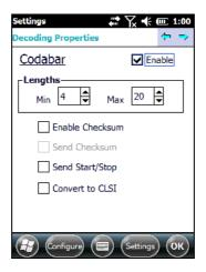
Codabar: Select Enable, Min/Max Lengths, Enable Checksum, Send Checksum, Send Start/Stop and Convert to CLSI.
