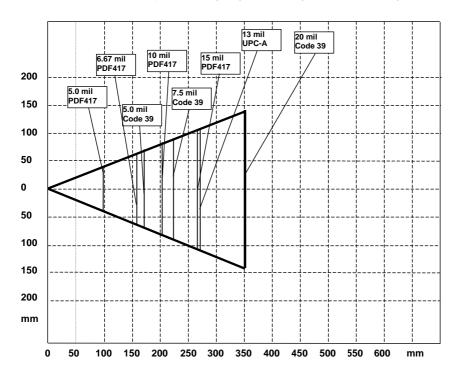
Typical Reading Diagram - Reading Zones (10° skew angle)
