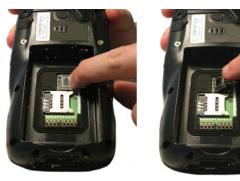
4. Insert the microSD card with the written part upward:
