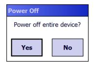
The user is given five seconds to respond. If the user selects "Yes", then the device, the cellular radio and GPS receiver are powered off. If the user selects "No", or does not respond within five seconds, the device will power off, but leave radios running as they were.
