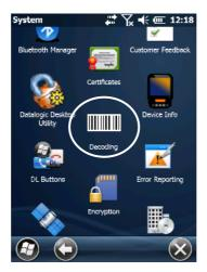
There are two sections in the Decoding control panel, each containing additional pages. There are seven General Configuration pages and multiple Barcode symbology pages.
