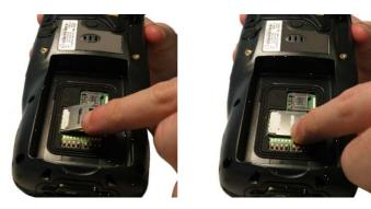
6. First insert the bottom and then the upper (contacts) side of the battery pack into the slot. First insert the bottom and then the upper (contacts) side of the battery pack into the slot. Press until the battery latch clicks twice.
