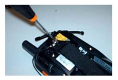
2. Lift the bottom of the hand strap to place the hook vertically:
