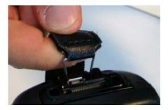
3. Press on the upper sides of the hook to remove it:
