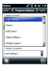
To configure the way up/down and the rest of keys control repeats, use the Up/Down Control page (Start > Settings > Personal > Buttons and tap Up/Down Control).
