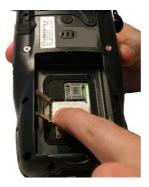
5. Lock the card into place by pushing the cardholder down and then shifting it to the right
