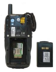
4. Install the new battery pack, first insert the bottom side, then the upper (contacts) side of the battery pack into the slot. Press until the battery latch clicks twice:
