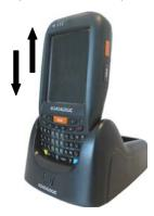
Figure 2 - Mobile Computer Insertion
