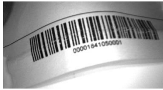
Figure 17 - Barcode Printed on Curved Surface Readable by Matrix 300N in spite of Image Optical Distortion
