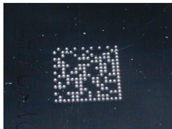
Figure 20 - Directly Marked Dot Matrix Code Characterized by Outstanding Separation Distance between Adjacent Code Elements
